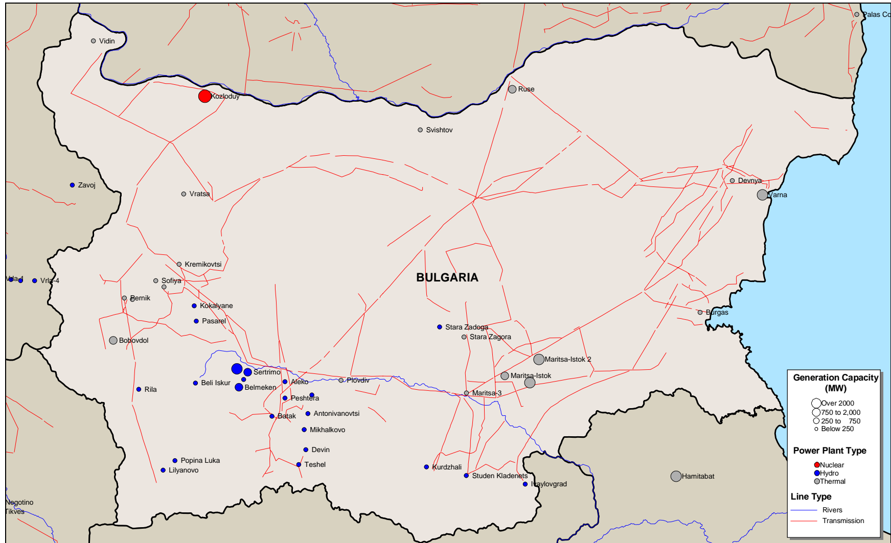
Figure 2. Bulgaria Electricity System Map.
